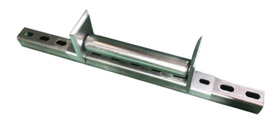
The Unistrut roller can be bolted directly down onto 42mm Unistrut (as illustrated above), flat plate or square box section up to 40mm. The roller can be made to any length but as standard comes in two sizes, 240mm (340mm overall length) and 175mm (275mm overall length).
