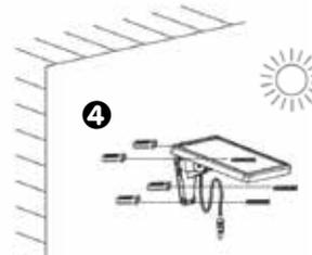
Use the holes on the mounting plate to mark out drill holes. Drill four holes, insert wall plugs and fix the mounting plate with screws. Rotate the solar panel so it is in direct sunlight.
