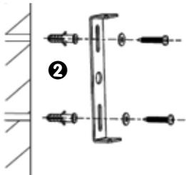
Use the holes on the mounting plate to mark the positions of the screws for drilling. Drill two holes in the mounting location, insert wall plugs and fix the mounting plate with screws.
