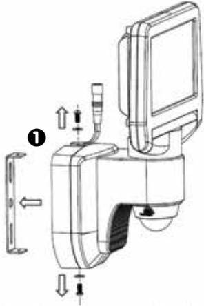
Loosen the two screws on the back of the main unit to release the mounting plate.
