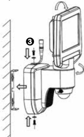
Use two screws to attached the floodlight back onto mounting plate.
