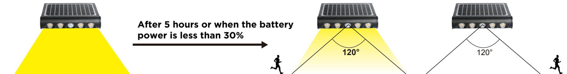
Lamp automatically lights up at night and keep 100% brightness, after 5 hours or when battery power is less than 30%, lamp turns to Energy Saving Mode: Lamp automatically turns to 100% brightness when motion is detected in the range  $\leq 8\text{mtrs}$ , then turns off after 20 seconds of no motion.
