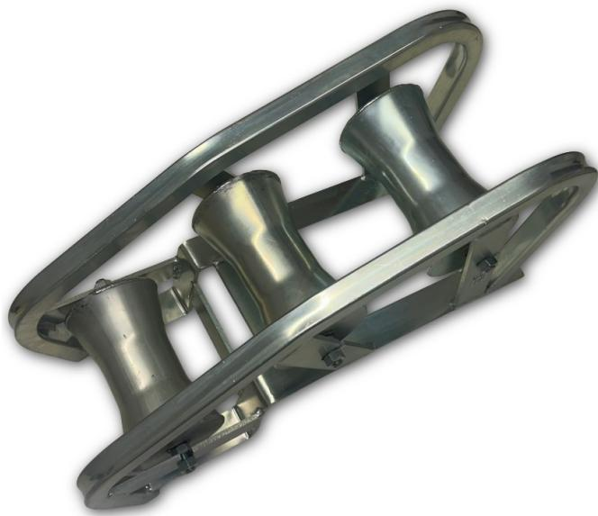
The manhole cable roller leads the cable from the drum into the jointbox/ manhole or the winch bond out of the manhole. This cable roller is suitable for cables of up to 130mm.
